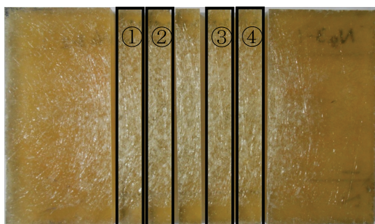
Fig.13 Photograph of specimens for bending test.
